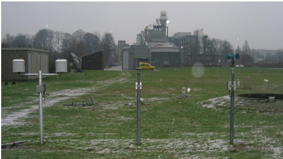
Figure 4: Instruments at the operational site DB260. To the left the KNMI multi-plate radiation shield for measuring temperature and to the right the cup anemometer. Both instruments operate at 1.5 m above ground level. The 4 parallel locations are equipped with the same instruments.
